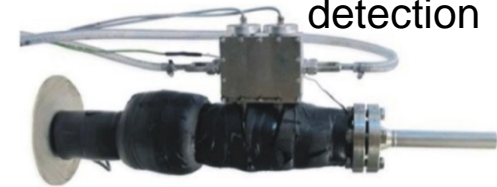
Microwave sensor for water and solids detection
