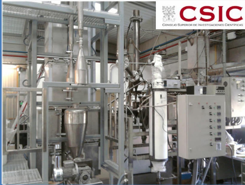
75 kW CSIC-ICB bubbling fluidized bed gasifier
