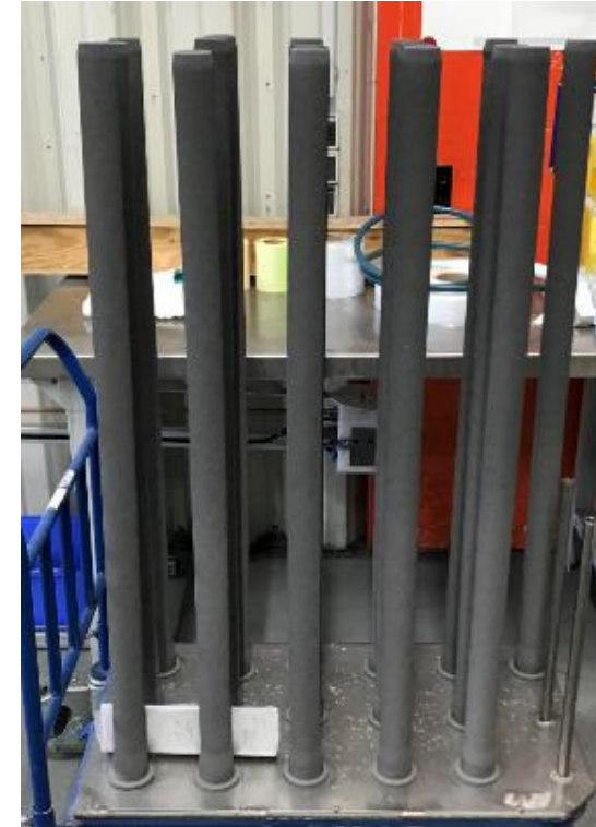
Heat treatment frame and delivered 1.2m filter elements
